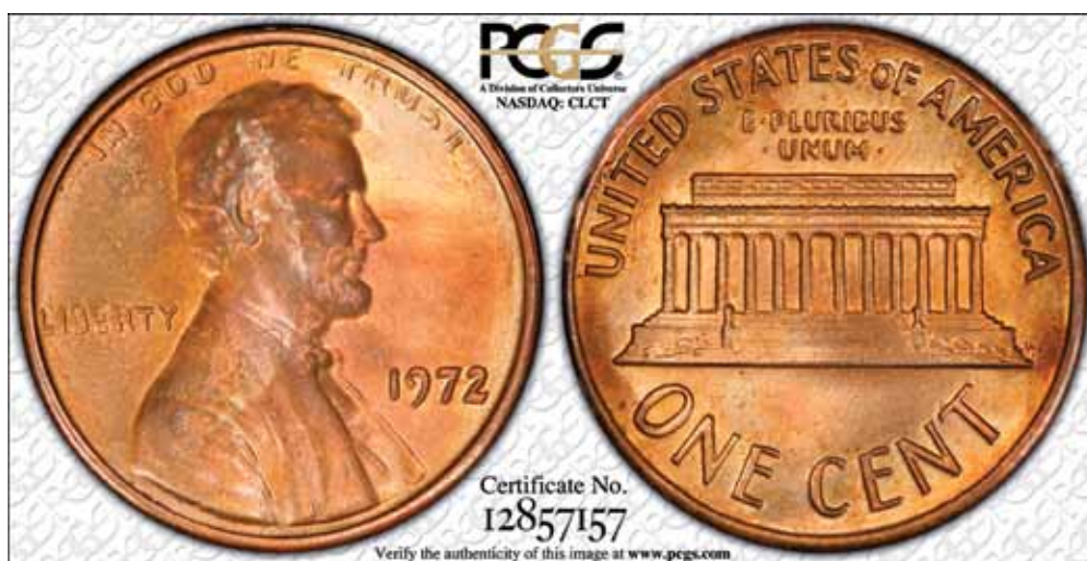
1972 DDO 1C Struck Counterfeit Rough fields and a raised lint mark on collar.
